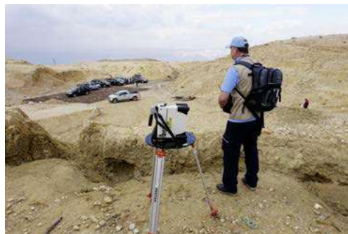
Gamma measurement on-site
