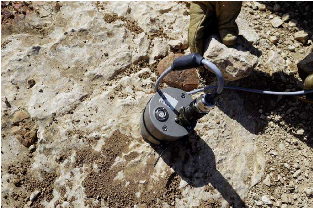
To localise tremors, seismic sensors were installed throughout the entire inspection area
