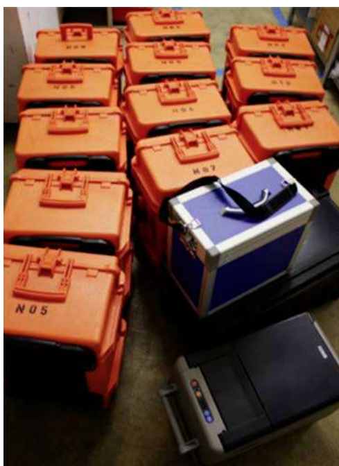
The mobile labs can be packed into 10 to 15 robust, dust and water tight boxes weighing 30 kg each for air or road transport
