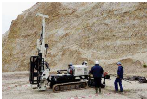
Subsoil-Gas-Sampling to measure various radioactive noble gases
