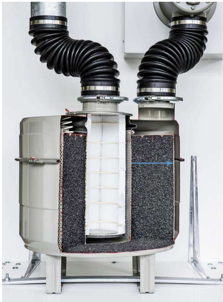
Sectional view of a big filter: The arrow indicates sorption bed depth and flow direction Sorption bed data: Volume: \geq 66 L Air flow rate: 150 \text{ m}^3/\text{h} Bed depth: 157 mm Flow velocity: 99 mm/s
