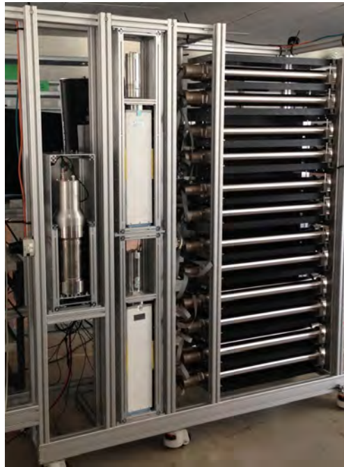
Series of neutron and gamma ray detectors on the manufacturer's test bench.
