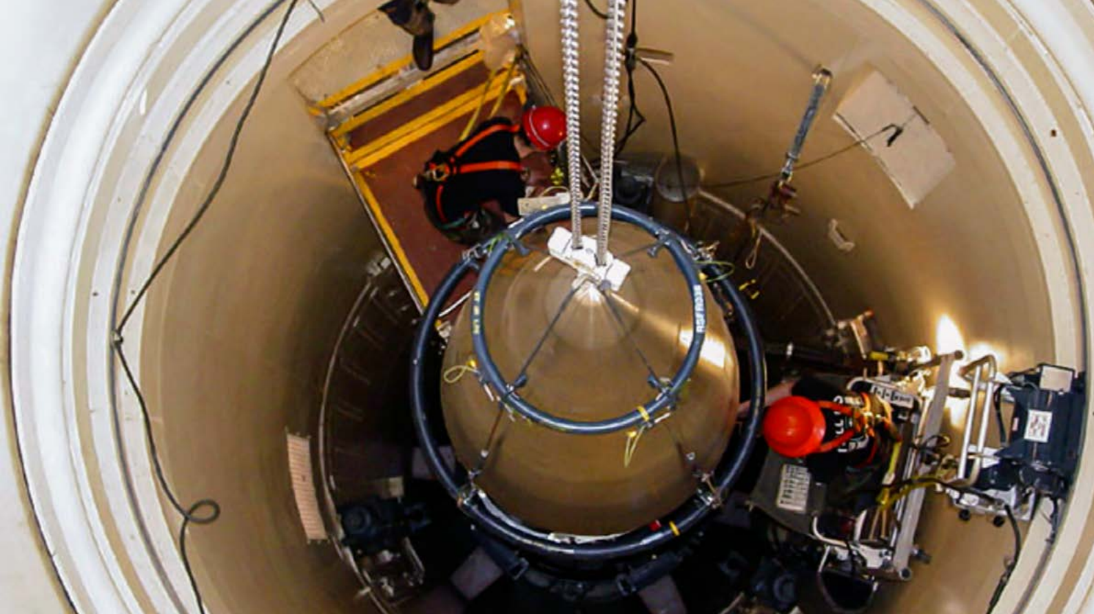
A US Air Force missile maintenance team removes the upper section of an intercontinental ballistic missile with a nuclear warhead in an undated USAF photo at Malmstrom Air Force Base, Montana.
